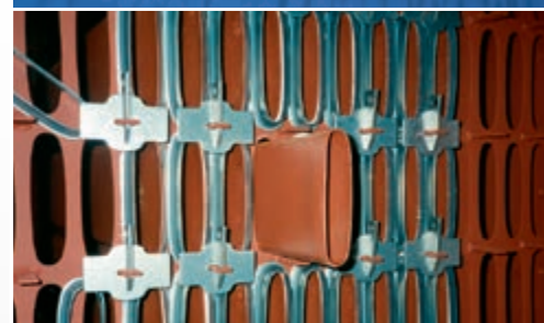
Perforated plate with flat-tube cooling elements
